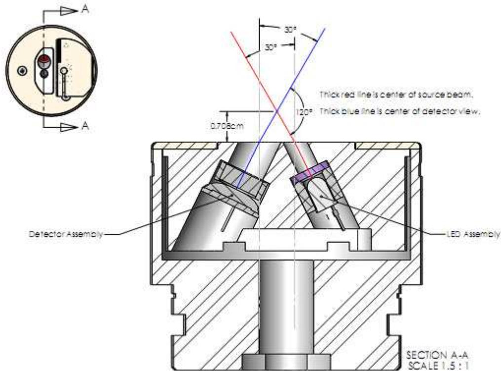
**Figure 1.** Optical configuration of *ECO* scattering meter
