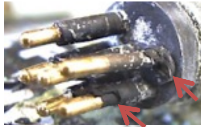
Material degraded "loose-sock effect"
