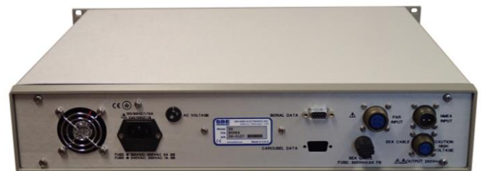
SBE 36 Deck Unit – back panel (connectors & fuses)
