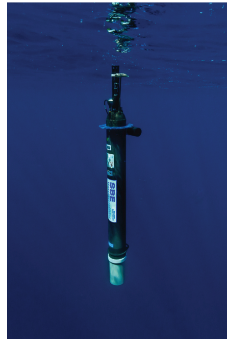
Navis BGC float 0028 after deployment. The ECO Triplet is visible on the upper right side of the float. Photo by Christopher Gerick.
